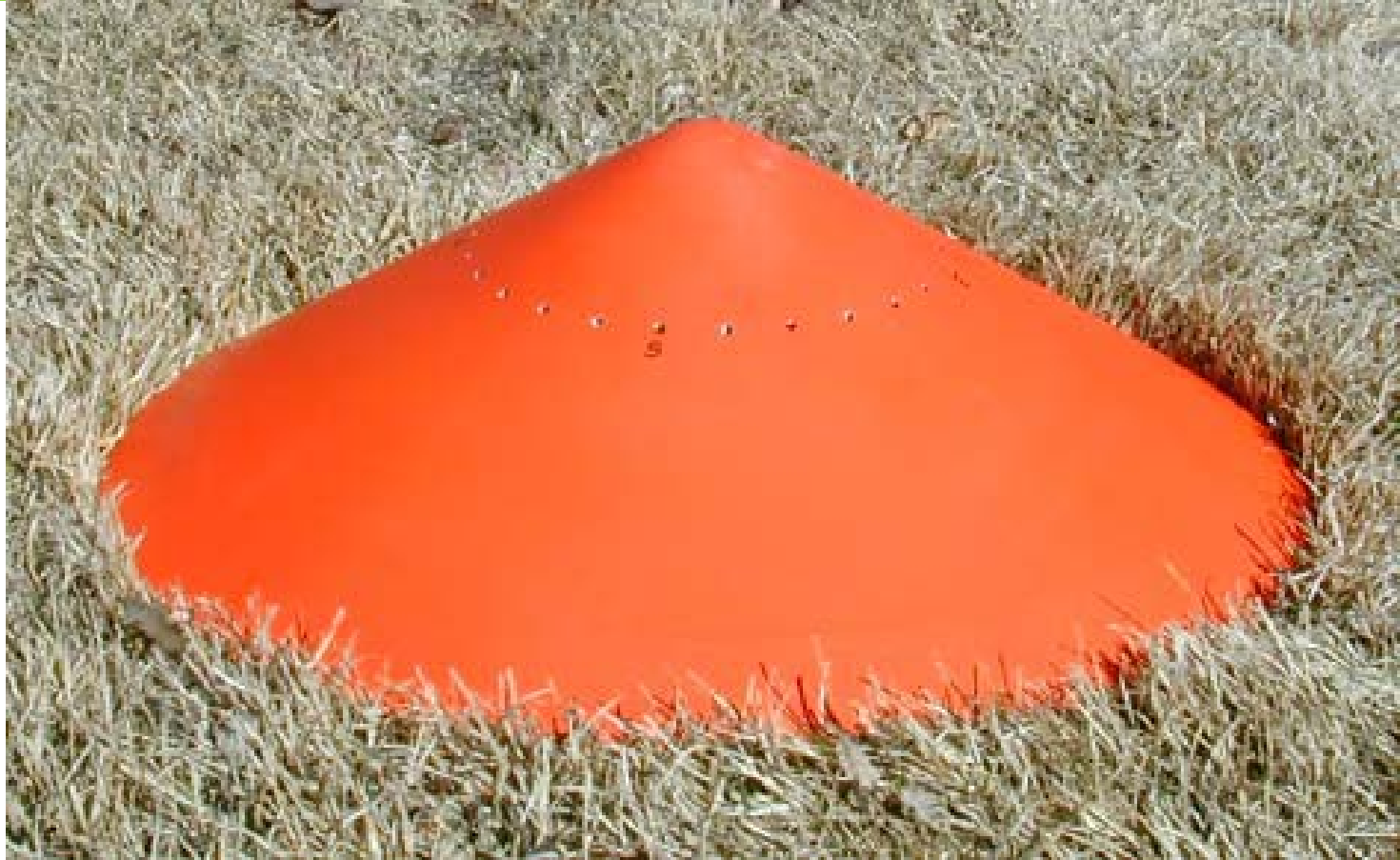
(a) Hardened In-Situ Tornado Pressure Recorder, HITPR [Karstens et al., 2010; Fig. 2; Samaras and Lee, 2004]
