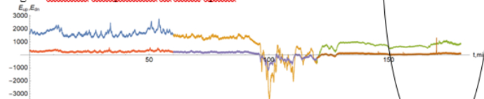
Fig. 4. Change in the magnitude of the electric field strength at two heights (0.4 and 5 m)
